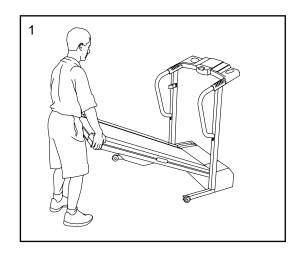
Move your right hand to the position shown and hold the treadmill firmly. Press out on the storage latch. Raise the treadmill until the storage latch closes over the catch. Make sure that the storage latch is fully engaged over the catch.
